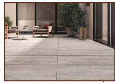
terraces, beaches, gardens, walkways and urban areas, Extragres 2.0 slabs can be dry-laid directly on sand, gravel and grassy ground so as to obtain a tiled area that can immediately withstand foot without requiring a screed and without the use of mortar and glues.
